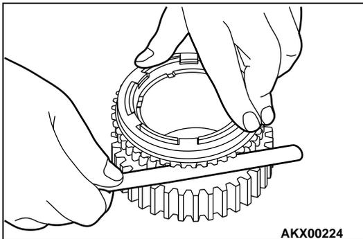
**>>L<< SYNCHRONIZER OUTER RING/SYNCHRONIZER CONE/SYNCHRONIZER INNER RING INSTALLATION**
