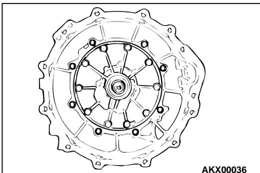
55. Install the converter housing.
