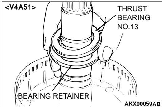
3. Install the bearing retainer and thrust bearing number 13 onto the output shaft. <V4A51>
