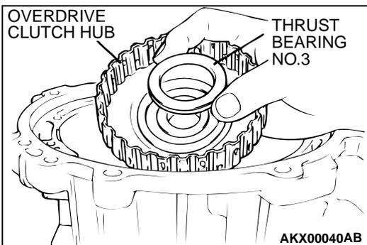
21. Remove the overdrive clutch hub and thrust bearing number 3.
