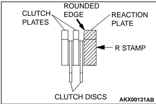
2. Install the reaction plate so that it is oriented as shown in the illustration. Assemble in the same manner as the clutch plate so the section with no teeth (A in the illustration) matches the retainer hole (B in the illustration).
