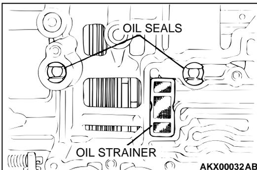
11. Remove the oil strainer and two oil seals.
