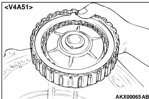
18. Install the underdrive clutch. <V4A51>
