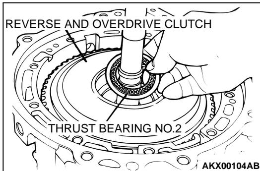
47. Install the reverse and overdrive clutch.
