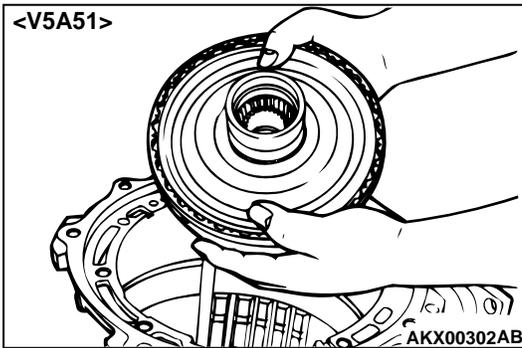
43. Remove the direct annulus gear. <V5A51>
