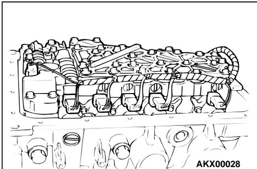
69. Connect the connector to the valve body.
