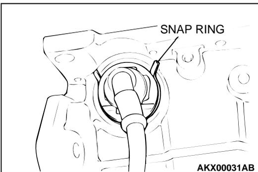
10. Remove the snap ring and disconnect the solenoid valve harness.
