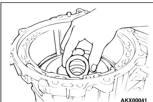
22. Remove the thrust bearing number 4.
