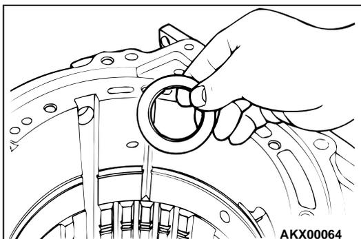
17. Apply vase line or petroleum jelly on the thrust bearing number 12, and then install on the front end of the output shaft <V4A51> or direct planetary carrier <V5A51>.
