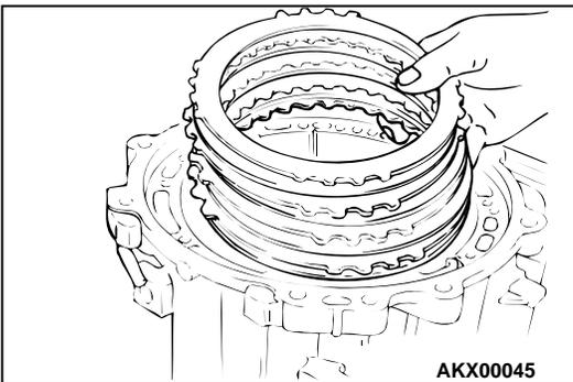
26.Remove the pressure plate, brake plate and brake disc.
