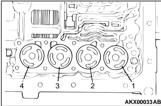
12. Remove each accumulator piston, seal ring, spring, snap ring <V5A51>, accumulator cover <V5A51>, O-ring <V5A51>.
