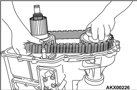
**>>N<< REAR OUTPUT SHAFT INSTALLATION**
