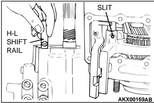
**>>E<< H-L SHIFT RAIL/SPRING PIN INSTALLATION**
