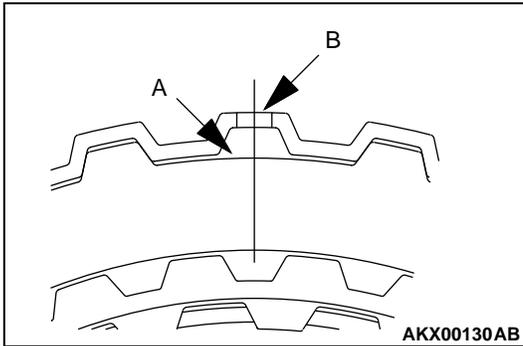
1. Alternately assemble the clutch plate and clutch disc in the reverse clutch retainer. Align and assemble both clutch plates (where there are no teeth) (A in the illustration) with the reverse clutch retainer hole (B in the illustration).
