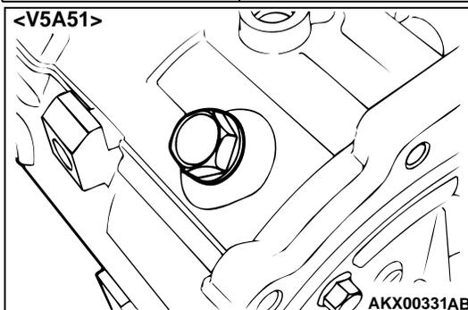
4. Install new O-ring on the anchor plug and tighten the anchor plug by specified torque. <V5A51>
