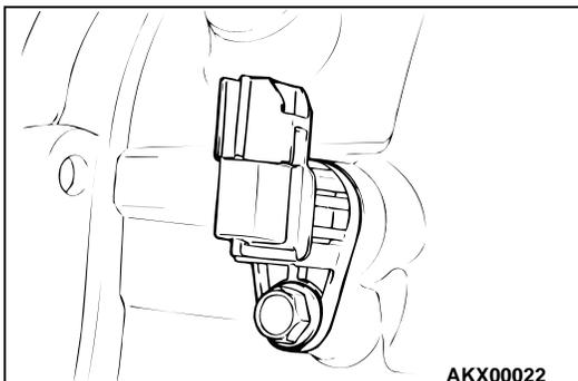
3. Remove the manual control lever, and then remove the park/neutral position switch.
