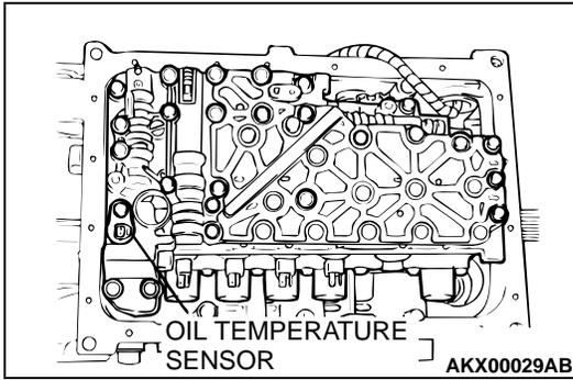
9. Remove the twenty valve body mounting bolts and then remove the valve body, O-ring and oil temperature sensor.
