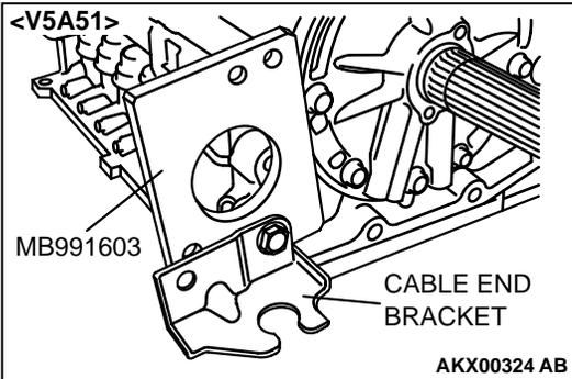
29. Using the Transfer case adapter bolt, install special tool MB991603.
