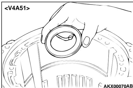
21. Apply Vaseline or petroleum jelly on the thrust bearing number 10, and then install it on the underdrive clutch hub. <V4A51>
