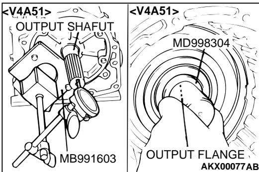
30. Select the thrust race number 8 with the following procedure:
