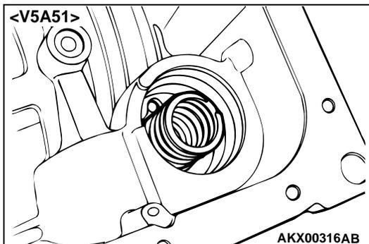
8. Install the reduction brake spring. <V5A51>
