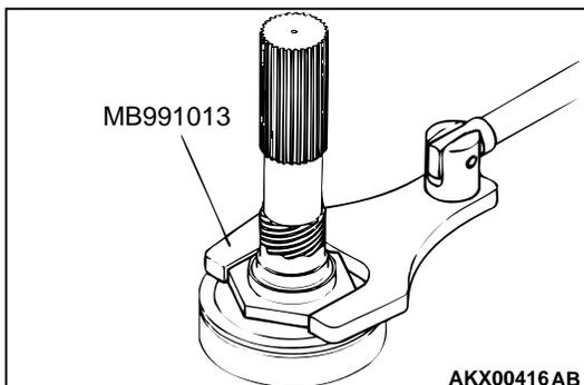
**<<C>> RADIAL BALL BEARING REMOVAL**
