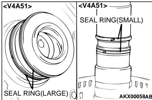
15. Install new seal rings (two large pieces and two small pieces) onto the output shaft <V4A51> or direct planetary carrier <V5A51>.
