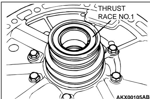
49. Apply Vaseline or petroleum jelly on the thrust race number 1 being used, and then install on the oil pump.
