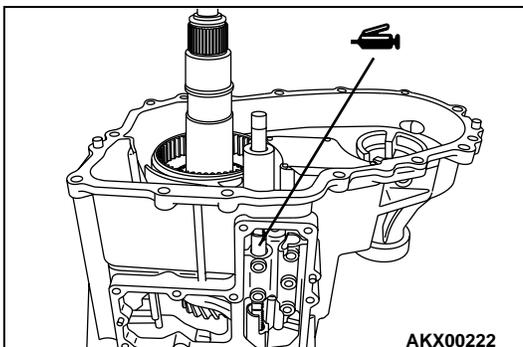
**>>J<< 2-4WD SHIFT FORK/2-4WD CLUTCH SLEEVE INSTALLATION**
