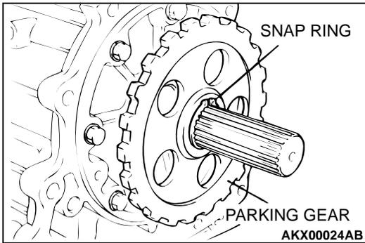
4. Remove the snap ring, and remove the parking gear using a puller [corresponding load approximately 9,800 N (2,200 pounds)].
