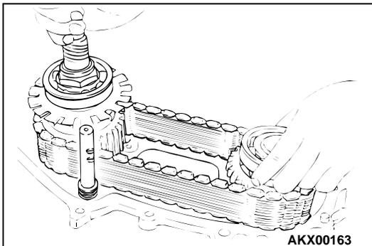
**ADJUSTMENT BEFORE ASSEMBLY****SPACER SELECTION FOR ADJUSTMENT OF COUNTERSHAFT GEAR END PLAY**
