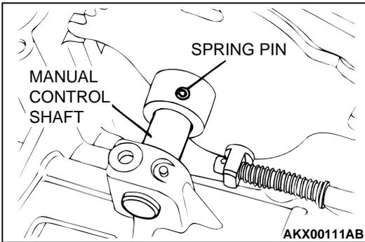
60. Hammer in so that the slit section of the spring valve is perpendicular to the axial direction of the manual control shaft.
