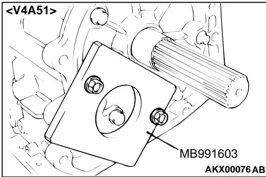
27. Remove the two output shaft support mounting bolts.
