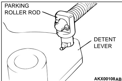
57. Install the parking roller rod to the detent lever.
