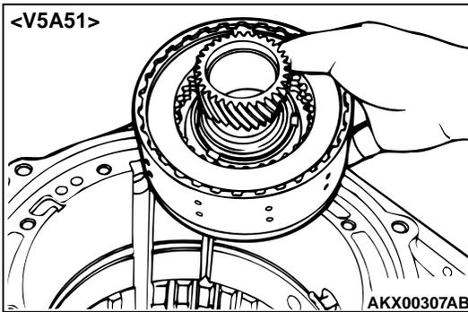
48. Remove the direct clutch. <V5A51>
