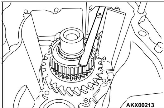
**>>E<< H-L SHIFT FORK/H-L CLUTCH SLEEVE INSTALLATION**
