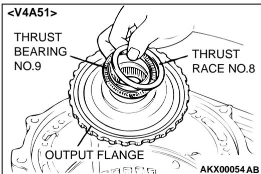
35.Remove the thrust race number 8, thrust bearing number 9 and output flange. <V4A51>
