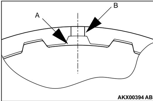
2. Install the reaction plate so that it is oriented as shown in the illustration. Assemble in the same manner as the clutch plate so that the section with no teeth (A in the illustration) matches the retainer hole (B in the illustration).
