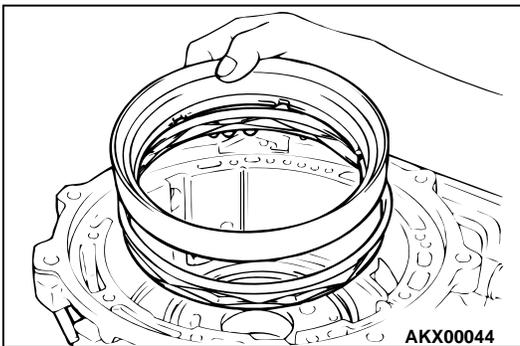
25.Remove the second brake and return spring.
