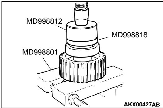
**>>B<< BALL BEARING INSTALLATION**
