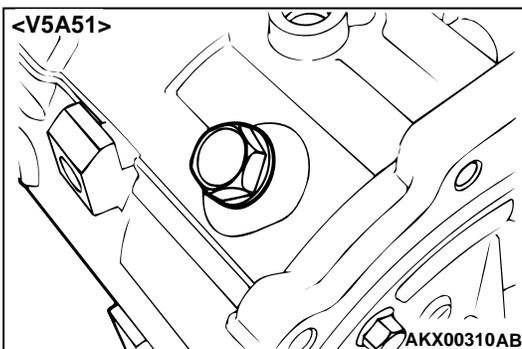
51. Remove the anchor plug and the O-ring. <V5A51>
