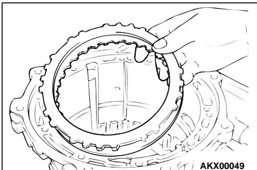
30. Remove the reaction plate and one brake disc.
