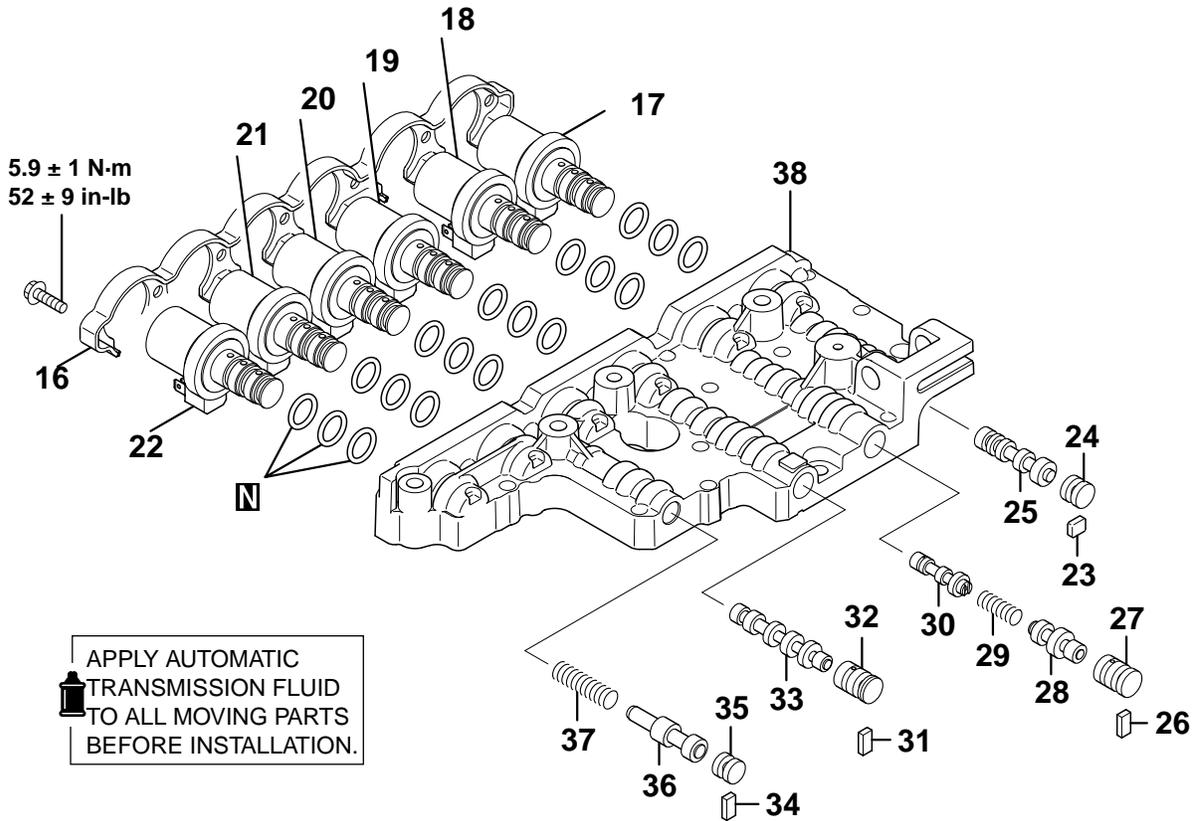
APPLY AUTOMATIC TRANSMISSION FLUID TO ALL MOVING PARTS BEFORE INSTALLATION.
