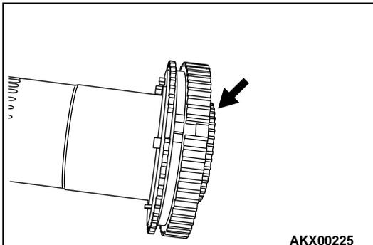
3. Combine the synchronizer outer ring, the synchronizer cone and the synchronizer inner ring, and install them by mating the notch of 2-4WD clutch hub and protrusion of the synchronizer outer ring.
