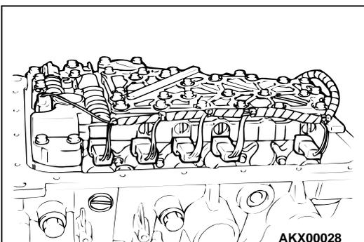
8. Disconnect the valve body harness connectors.
