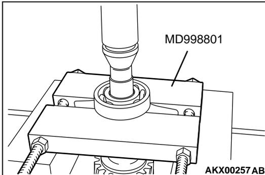
**<<B>> SPACER/ROLLER BEARING/INNER RACE REMOVAL**
