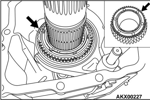
2. Install the chain, the drive sprocket and the front output shaft onto the transfer case in combined state.
