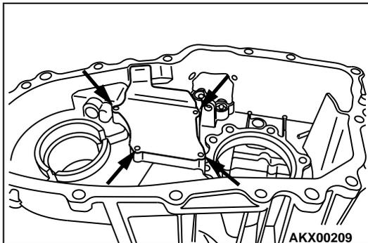
**ASSEMBLY SERVICE POINTS****>>A<< OIL GUIDE INSTALLATION**
