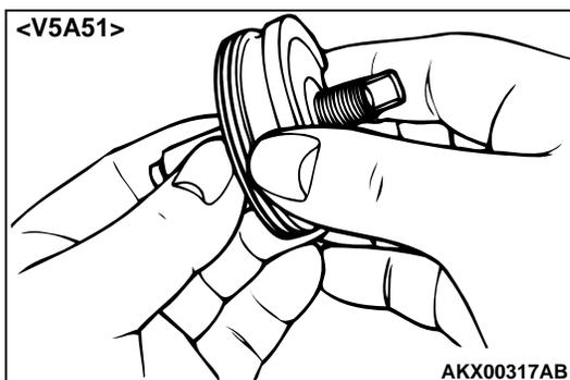
9. Tighten the reduction brake piston adjust rod into the reduction brake piston manually to the full. <V5A51>
