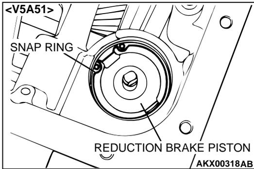
11. Press the reduction brake piston into the transmission case, and then install the snap ring. <V5A51>
