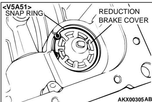
46. Remove the snap ring and then the reduction brake piston cover and O-ring. <V5A51>
