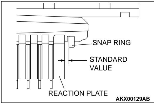
3. Confirm that the clearance (overdrive clutch end play) of the snap ring and reaction plate is the standard value. If the clearance is not at the standard value, select the snap ring and adjust so that the clearance is within the standard value.
