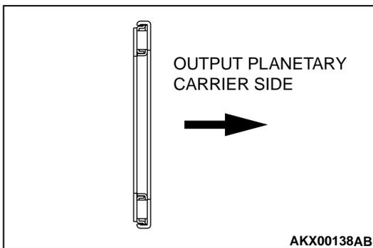
**>>C<< THRUST BEARING NUMBER 6 INSTALLATION**
