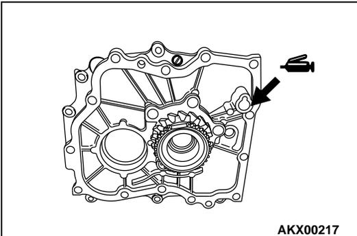
2. Face the notched section of the input gears in the direction shown in the illustration.
