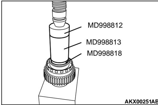
**>>B<< BALL BEARING INSTALLATION**
