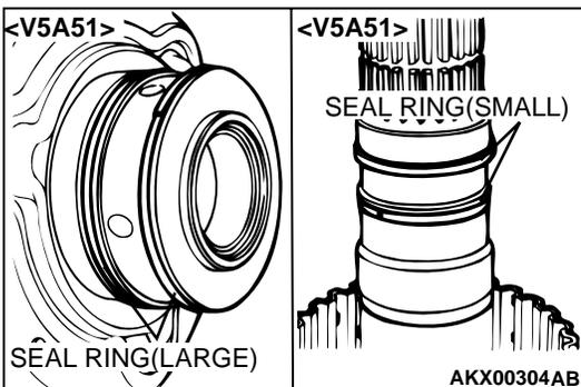
45. Remove the two large and two small seal rings from the direct planetary carrier. <V5A51>
