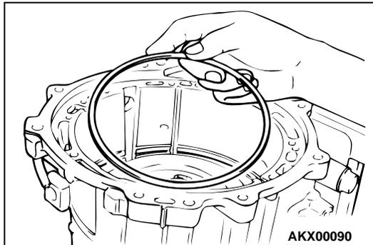
36. Install the wave spring to the low/reverse brake piston.
