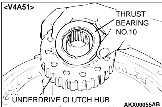
36.Remove the thrust bearing number 10 and underdrive clutch hub. <V4A51>
