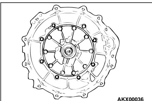
15. Remove the eight converter housing mounting bolts, and then the converter housing.
