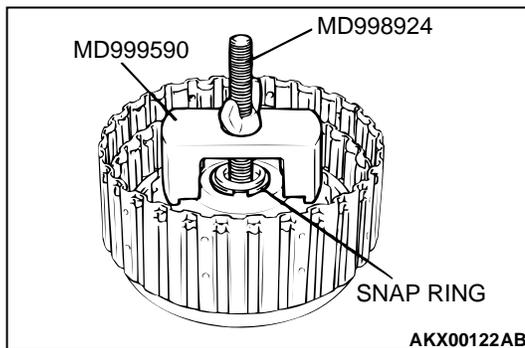
**ASSEMBLY SERVICE POINTS****>>A<< D-RING INSTALLATION**
