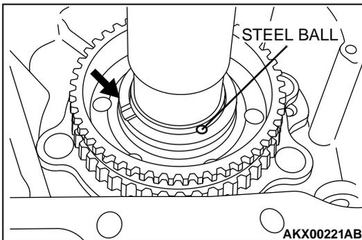
**>>I<< STEEL BALL/SPACER INSTALLATION**
