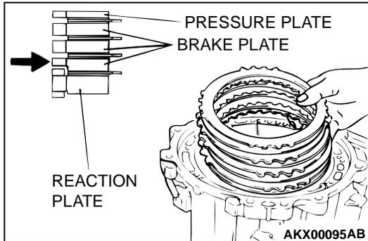
41. Install the brake disc, brake plate and pressure plate selected in step 32 (9).
