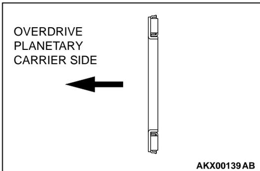
**>>D<< THRUST BEARING NUMBER 5 INSTALLATION**
