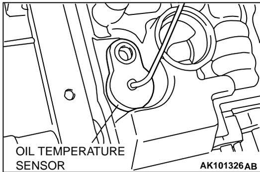
68. Install the oil temperature sensor.
