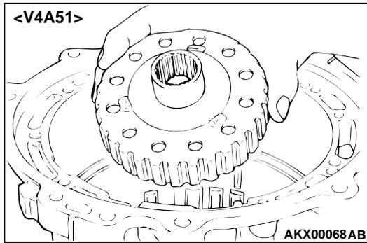
20. Install the underdrive clutch hub. <V4A51>
