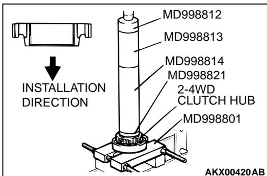
**>>C<< BALL BEARING INSTALLATION**
