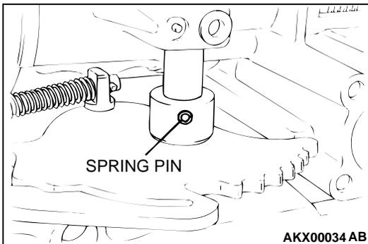
13. Remove the detent lever spring pin.
