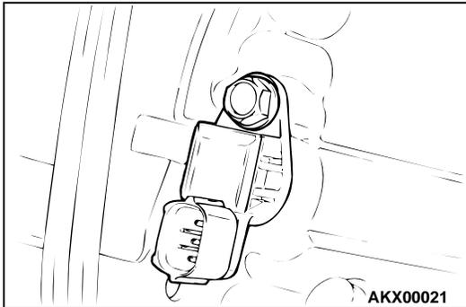
2. Remove the output shaft speed sensor.
