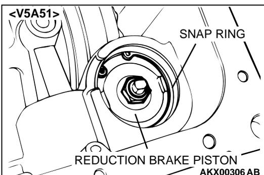
47. Remove the snap ring and then the nut, reduction brake piston, seal ring. Adjust rod and spring. <V5A51>
