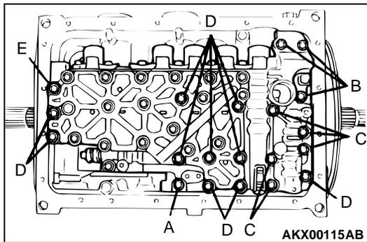
67. Tighten the twenty valve body mounting bolts to the specified torque.
