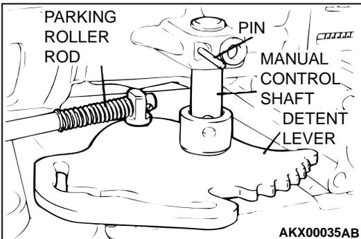
14. Remove the pin, and then remove the manual control shaft, two O-rings, detent lever and parking roller rod.
