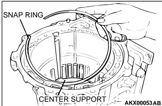
34.Remove the snap ring and center support.
