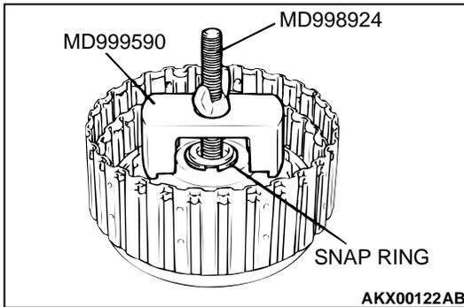
**>>E<< CLUTCH PLATE/CLUTCH DISC/REACTION PLATE INSTALLATION**
