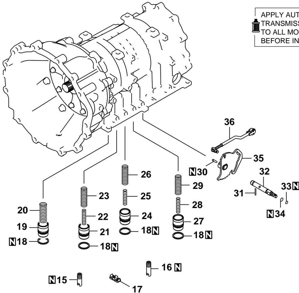
APPLY AUTOMATIC TRANSMISSION FLUID TO ALL MOVING PARTS BEFORE INSTALLATION.
