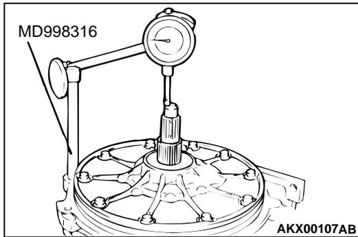
52. Using special tool MD998316, set a dial gauge as shown in the illustration. Measure the end play of the input shaft, and select the thrust race installed in step 36 so that the end play is at the standard value. Then, reassemble.
