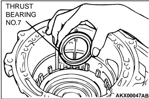
28. Remove the thrust bearing number 7.
