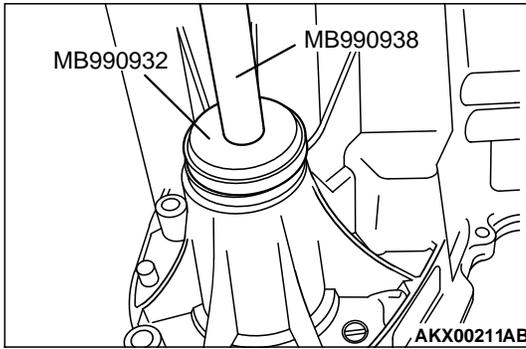
**>>C<< REAR BEARING RETAINER INSTALLATION**
