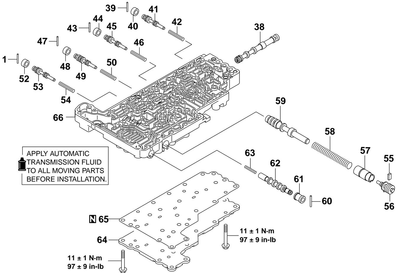
APPLY AUTOMATIC TRANSMISSION FLUID TO ALL MOVING PARTS BEFORE INSTALLATION.
