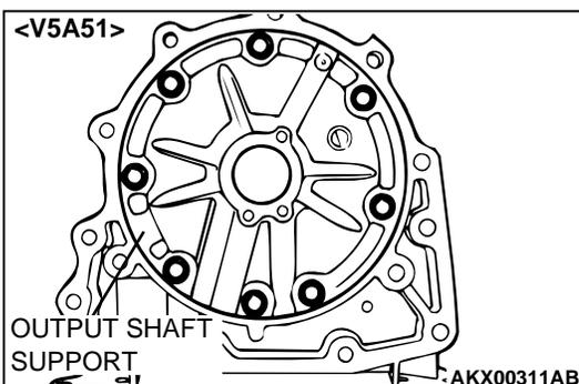
52. Remove the eight output shaft support mounting bolts, and then remove the output shaft support and gasket. <V5A51>
