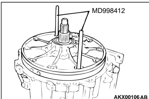
50. Install special tool MD998412 at the position shown in the illustration, and using this as a guide, install the oil pump and gasket.
