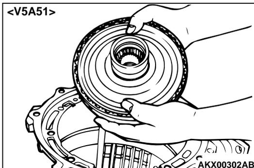
24. Apply Vaseline or petroleum jelly on the thrust bearing number 9, and then install on the output flange <V4A51> or direct annulus gear <V5A51>.
