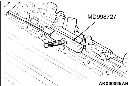
5. Remove the twenty oil pan mounting bolts and then using the special tool MD998727 to remove the oil pan.
