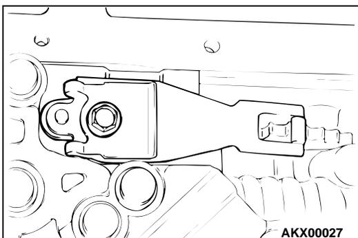
7. Remove the detent spring.
