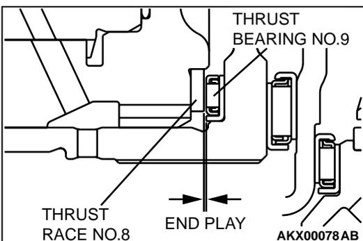
31. Using the following steps, select the snap ring for fixing the center support.
