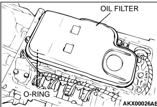
6. Remove the oil filter and O-ring.
