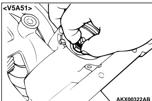
(3) Remove the special tool and tighten the reduction brake piston nut manually.
