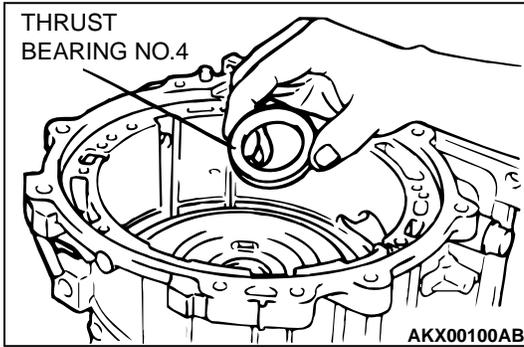
44. Apply Vaseline or petroleum jelly on the thrust bearing number 4, and then install on the reverse sun gear.
