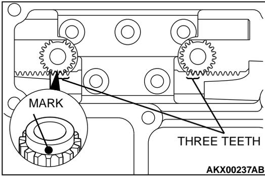
**>>U<< SHIFT RAIL DRIVE GEAR INSTALLATION**
