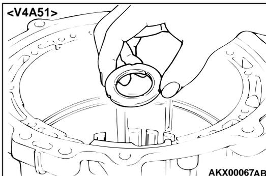
19. Apply Vaseline or petroleum jelly on the thrust bearing number 11, and then install on the front end of the underdrive clutch retainer. <V4A51>
