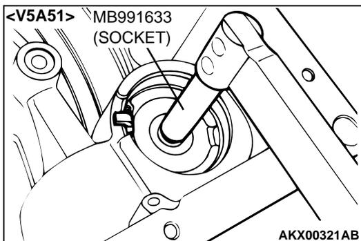
(2) Mount the torque wrench to the special tool (Socket), and after repeatedly tightening and turning back with the torque of 9.8 N·m (87 in - lb) twice, tighten the reduction brake piston adjust rod by the specified torque of 4.9 N·m (44 in - lb). Then turn the reduction brake piston adjust rod 5 1/2 to 5 3/4 turns backwards.
