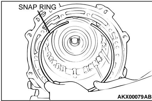
(2) After pushing the output shaft <V4A51> or direct planetary carrier <V5A51>, and the center support in alternately, and then measure the end play of center support.
