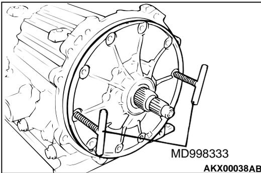
18. While screwing in special tool MD998333 evenly, remove the oil pump.
