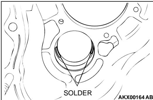
4. Using a micrometer, measure the thickness of the crushed solder. Based on the result, select a spacer which adjusts the end play to the standard value shown below:
