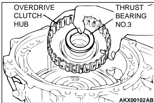
45. Apply Vaseline or petroleum jelly on the thrust bearing number 3, and then install on the overdrive clutch hub.
