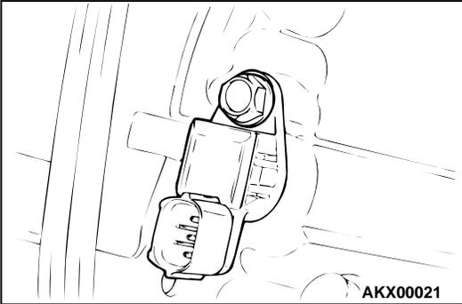
80. Install the input shaft speed sensor.
