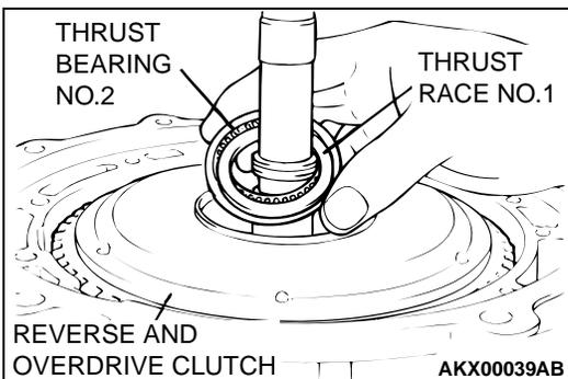
20. Remove the reverse and overdrive clutch, thrust race number 1 and thrust bearing number 2.
