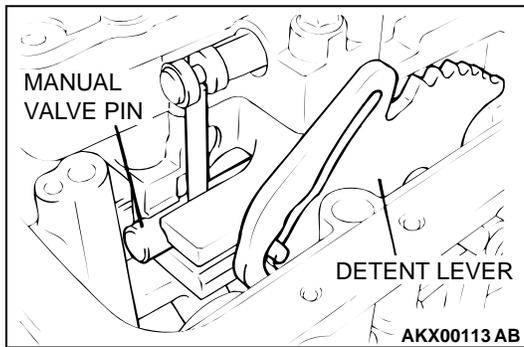
66. Install the valve body while inserting the manual valve pin into the detent lever groove.
