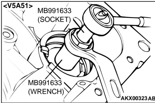
(4) Tighten the reduction brake piston nut to the specified torque using the special tool (wrench) with the special tool (Socket) so it does not rotate.
