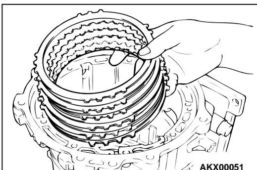
32. Remove the brake plate, brake disc, and pressure plate.
