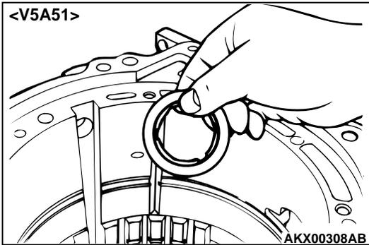
49. Remove the thrust bearing number 13. <V5A51>
