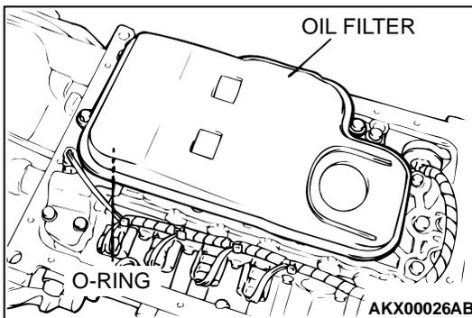
72. Install the oil filter and a new O-ring.
