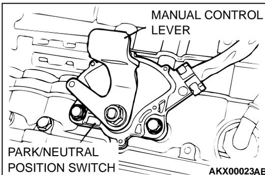
78. Install the park/neutral position switch and manual control lever.
