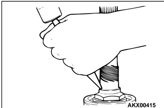
4. Use special tool MB991013 to remove the jam nut.
