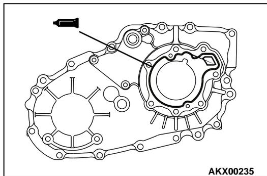
**>>T<< MAIN SHIFT RAIL/SHIFT ACTUATOR INSTALLATION**
