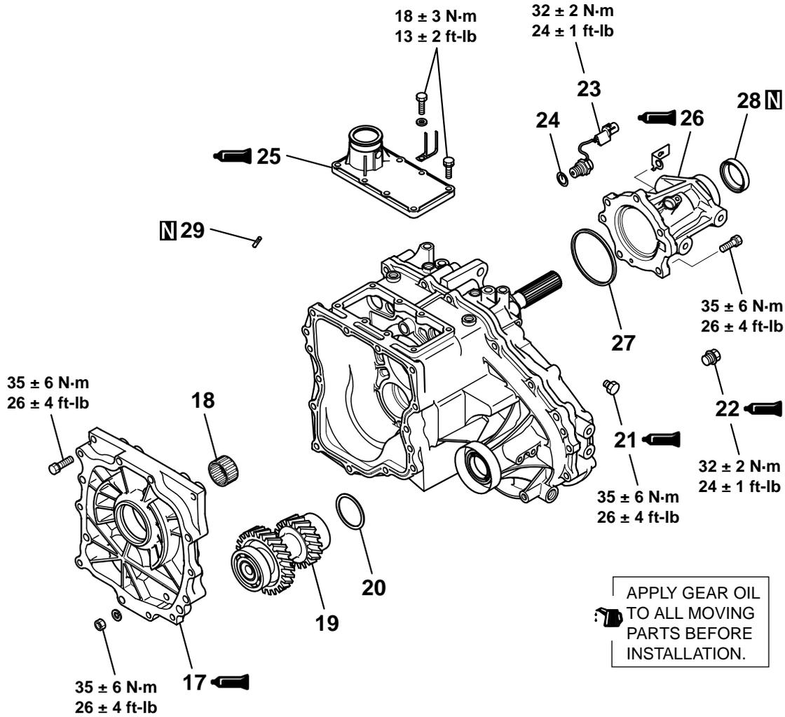
APPLY GEAR OIL TO ALL MOVING PARTS BEFORE INSTALLATION.
