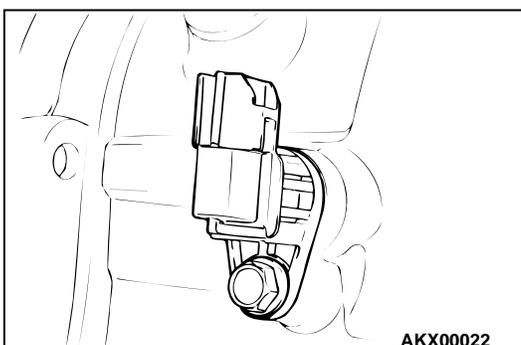
79. Install the output shaft speed sensor.
