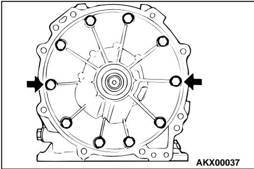
16. Remove the ten oil pump mounting bolts.
