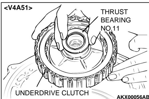
37.Remove the thrust bearing number 11 and underdrive clutch. <V4A51>
