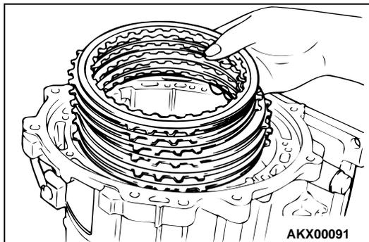
37. Install the pressure plate, brake disc and brake plate selected in step 32 (12).
