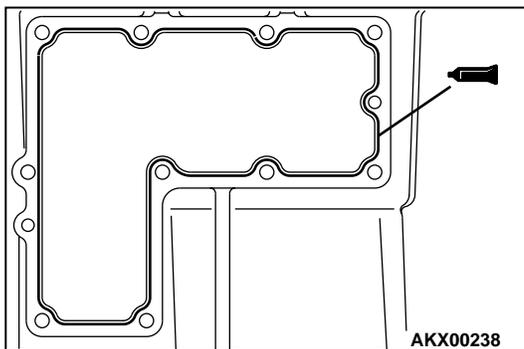
**>>W<< 2-4WD DETECTION SWITCH/4H DETECTION SWITCH/CENTER DIFFERENTIAL LOCK DETECTION SWITCH/2WD DETECTION SWITCH/4LLC DETECTION SWITCH INSTALLATION**
