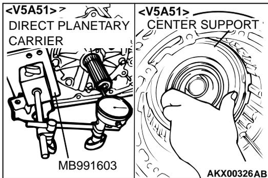
(3) Select the snap ring for fixing the center support installed in step 31 (1) so that the end play of the center support is at the standard value. Then, reassemble.
