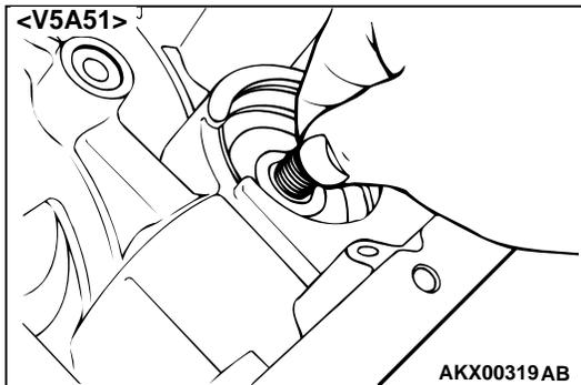
12. Fully tighten the reduction brake piston adjust rod manually. <V5A51>
