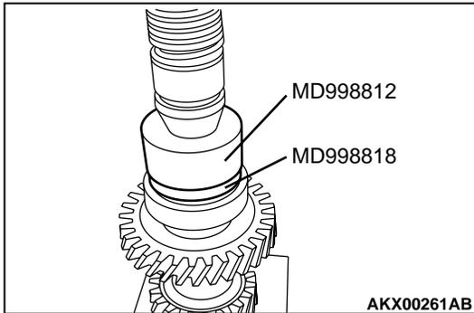
**>>C<< BALL BEARING INSTALLATION**
