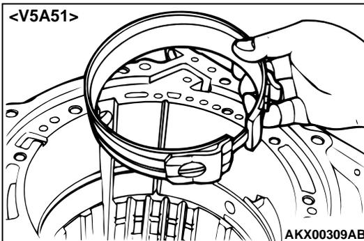
50. Remove the reduction brake band. <V5A51>
