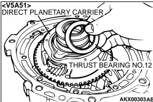
44. Remove the thrust bearing number 12 and direct planetary carrier. <V5A51>
