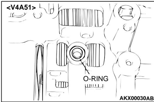
65. Install the new O-ring into the transmission case at the position shown in the illustration.
