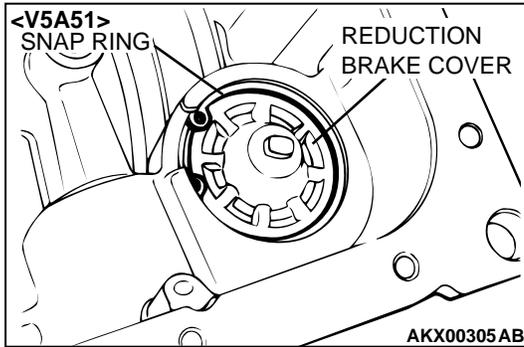
14. Install a new O-ring on the reduction brake piston cover, and then install the cover and the snap ring on the transmission case. <V5A51>
