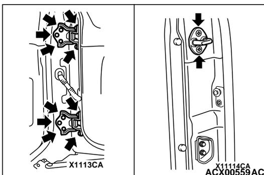
1. If the striker and latch mesh badly, move the striker forward and backward or right and left to adjust.
