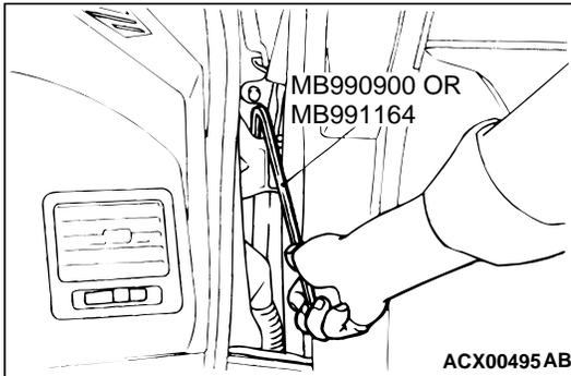
1. Use special tool MB990900 or MB991164 to loosen the hinge mounting bolts on the body side, and then adjust the clearance around the door so that it is uniform on all sides.
