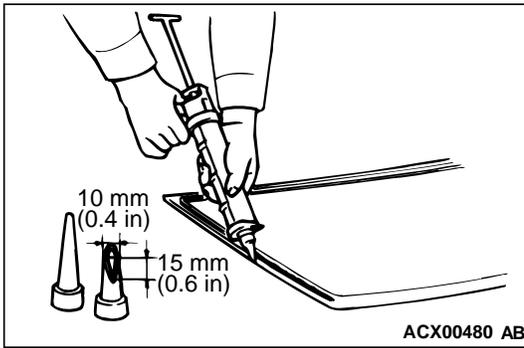
7. Fill a sealant gun with adhesive. Then apply the adhesive evenly around the windshield within 30 minutes after applying the primer.
