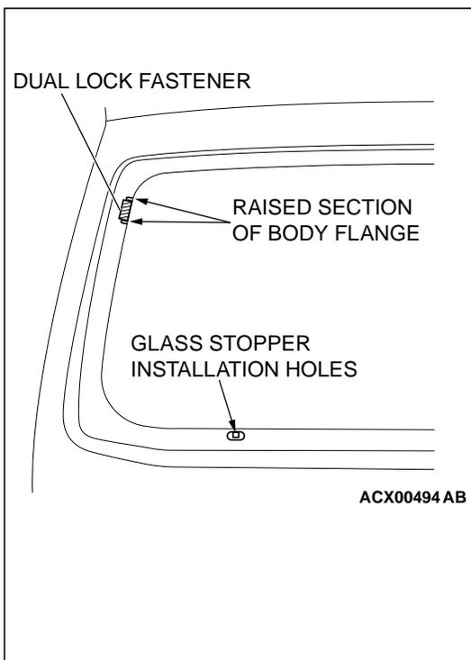
3. Attach the dual lock fastener at the specified position on the body flange.
