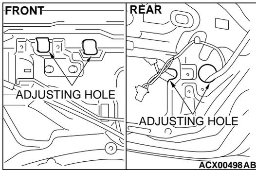
3. Fully close the door window glass again and tighten the door glass mounting screw firmly via the adjusting hole.
