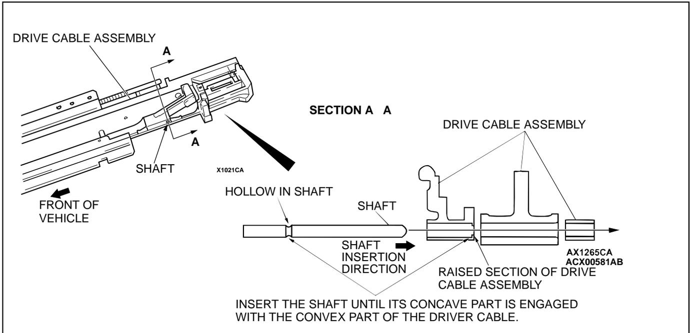
Install the shaft to the drive cable from the outside of vehicle as shown in the illustration.
