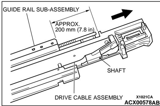
**<<B>> ROOF WINDOW DEFLECTOR PANEL ASSEMBLY REMOVAL**
