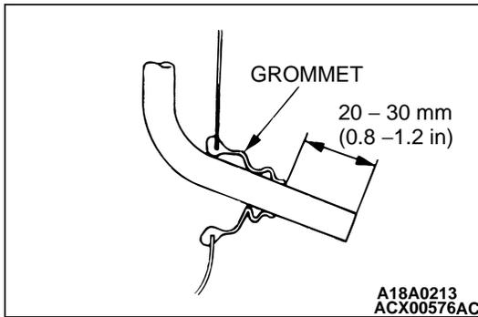
3. Install the grommet, and then position the drain hose so that it protrudes from the grommet as shown in the illustration.
