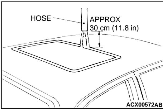
3. Hold the end of the hose approximately 30 cm (11.8 inches) above the roof and let the water run onto the weatherstrip for 5 minutes or more.
