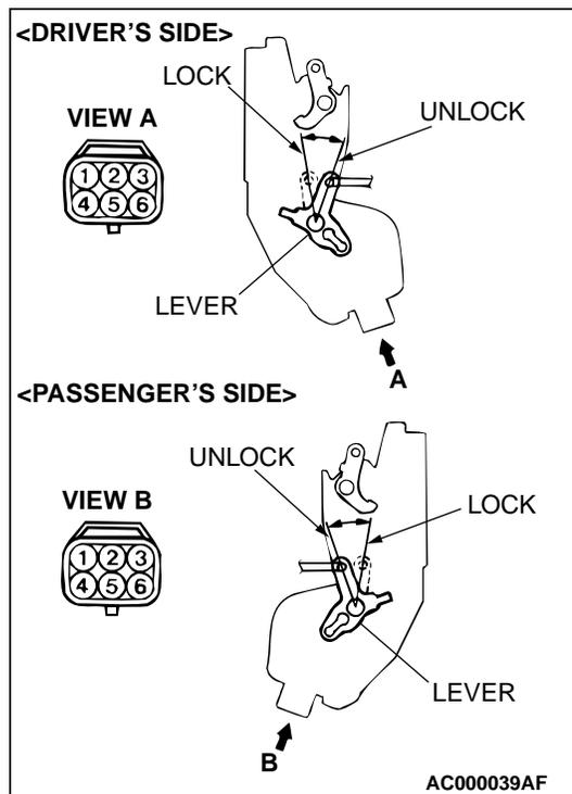
**Actuator Switch Check <Driver's side>**
