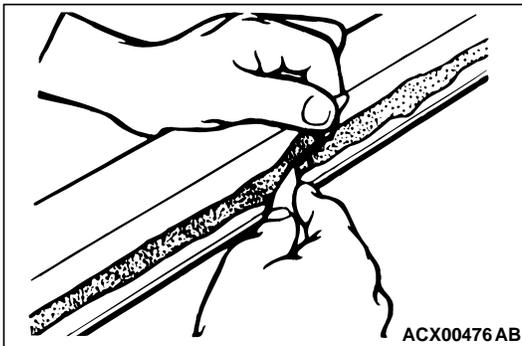
2. Using a sharp-point drill, make a hole in the windshield adhesive.
