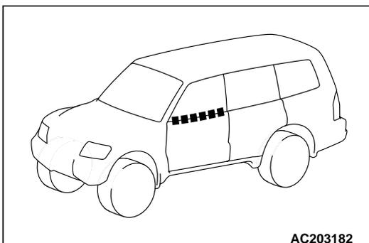
1. Attach cloth tape to every place, such as panel seams, projections, molding seams, glass and body seams, etc. which might conceivably be the source of wind noise.
