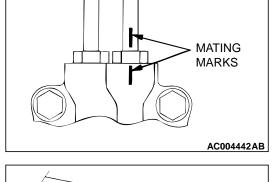
2. Connect the return pipe so that the marking is positioned as shown in the illustration.
