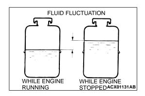
4. Check the difference of the fluid level when the engine is stopped, and while it is running. If the change of the fluid level is 5 mm (0.2 inch) or more, air bleeding should be done.
