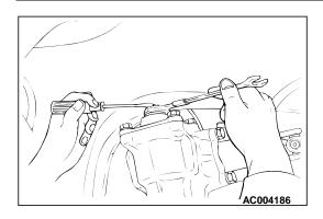
4. If the measured value exceeds the limit, screw in the steering gear box adjusting bolt until the steering wheel free play is within the standard value.
