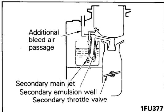
**INSPECTION OF SECONDARY WELL BLEED NIPPLE FOR CLOGGING—<sup>N14FRBB</sup>High altitude specifications for the 49 states only (excluding California)**
