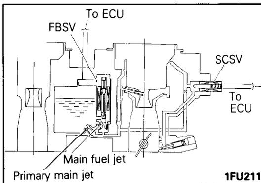
When the FBSV is energized, the main fuel jet is closed to leave the primary main jet passage as the only fuel passage. This will reduce the amount of fuel, resulting in leaner air-fuel mixture.
