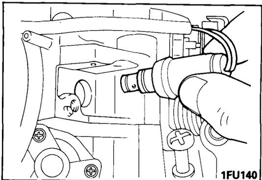
**25. REMOVAL OF SLOW CUT SOLENOID VALVE (SCSV)**
