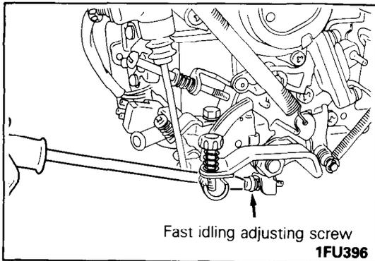
(5) Start the engine and check the fast idle speed.
