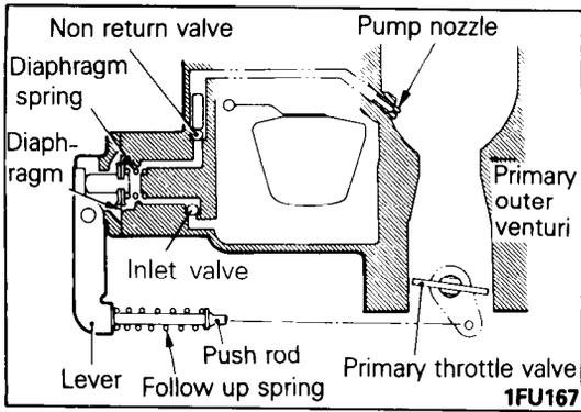
**INSPECTION OF CARBURETOR ACCELERATION PUMP**
