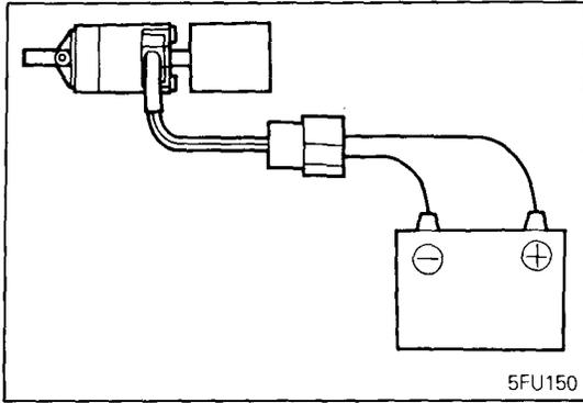
(4) Apply vacuum and check air tightness for both when battery voltage is directly applied to the solenoid valve terminal and when no voltage is applied.
