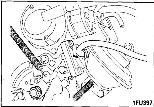
(7) Connect the vacuum hose removed in step (3) to the choke opener and check that the choke opener cancels fast idle.
