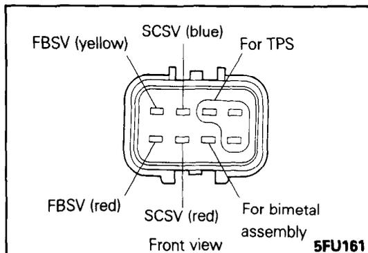
**25. INSTALLATION OF SLOW CUT SOLENOID VALVE (SCSV)/20. FEEDBACK SOLENOID VALVE (FBSV)**
