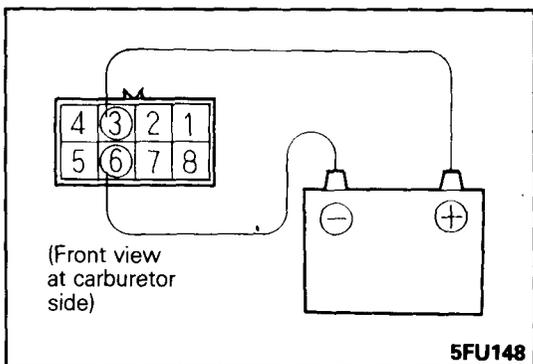
**SIMPLE INSPECTION OF SLOW CUT SOLENOID VALVE (SCSV)**
