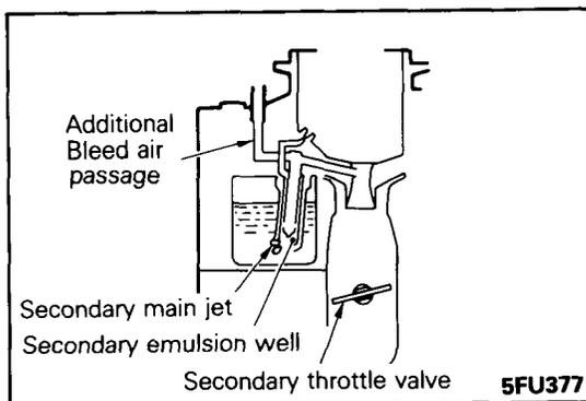
**Inspection for Clogging of Secondary Well Bleed Nipple – High altitude specifications for the 49 states**
