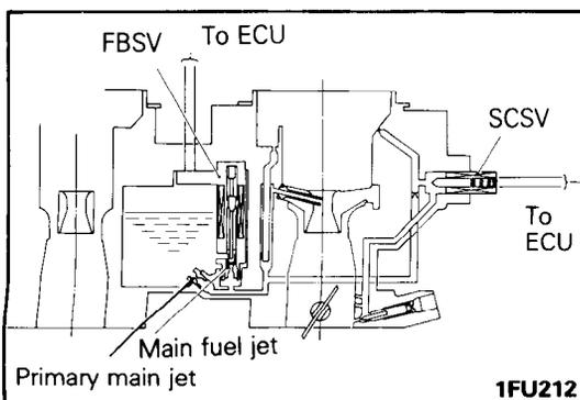
When FBSV is de-energized, the main fuel jet is opened to provide two fuel passages including the primary main jet passage. Since this will increase the amount of fuel, richer air-fuel mixture is obtained.
