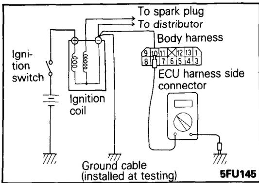
**INSPECTION OF ENGINE SPEED SENSOR (IGNITION COIL ⊖ TERMINAL)**
