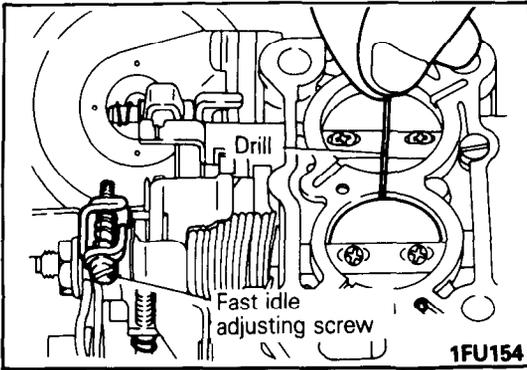
(2) Measure the primary valve to throttle bore clearance.
