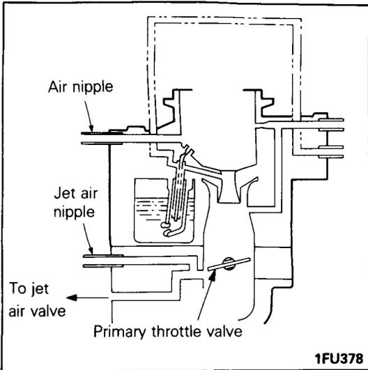
**INSPECTION OF JET AIR NIPPLE FOR CLOGGING—High altitude specifications for the 49 states (excluding California) only**
