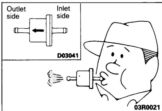
**CHECKING OVERFILL LIMITER (TWO-WAY VALVE)**
