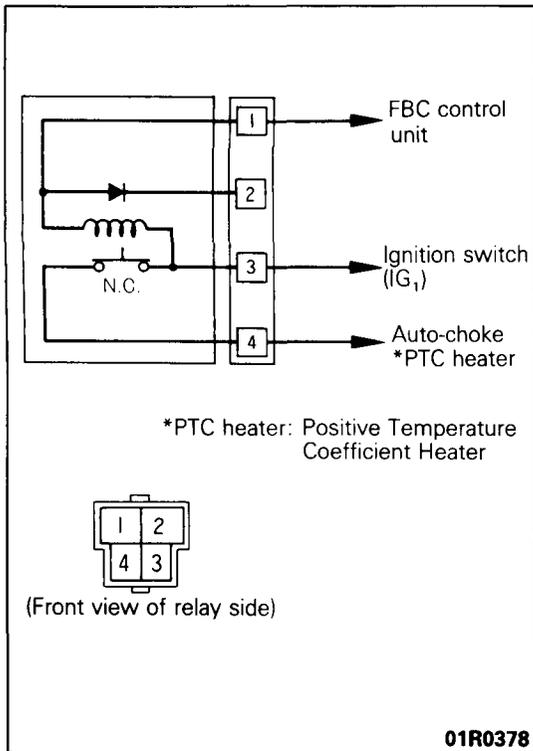
(2) Check for continuity between terminals when there is and is not current flow to the relay coil.
