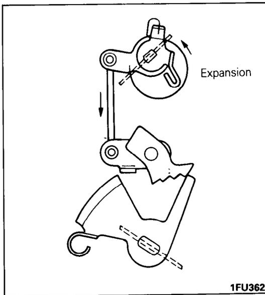
4. Shortly after starting of engine, the bimetal is heated by the heater and expands to open the choke valve gradually and push down the stopper lever. At this time, the engine speed increase gradually.
