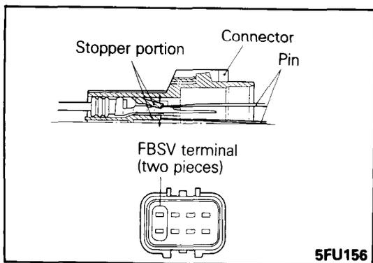
**20. REMOVAL OF FEEDBACK SOLENOID VALVE (FBSV)**
