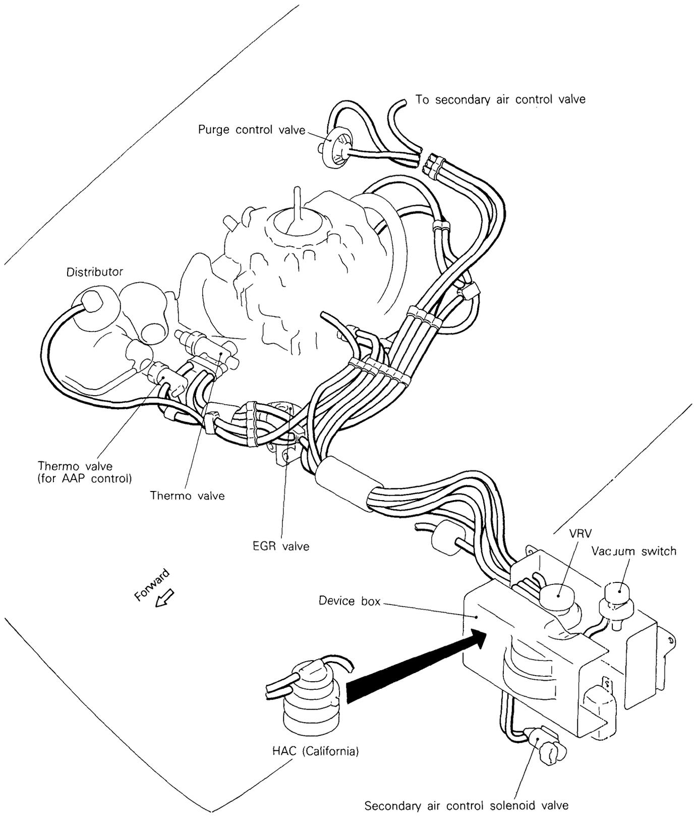
**INSPECTION OF THROTTLE OPENER CONTROL SYSTEM FOR AIR CONDITIONER LOAD**
