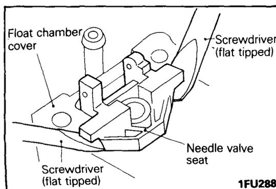
**16. REMOVAL OF NEEDLE VALVE SEAT**
