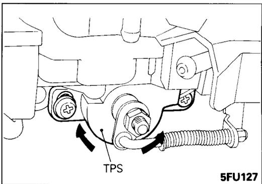
2. At this time, the fast idle control should have been released (the lever not resting on the fast idle cam).
