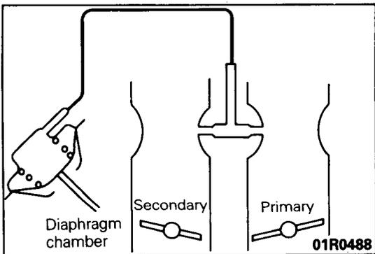
**INSPECTION OF CARBURETOR SECONDARY VALVE OPERATION**
