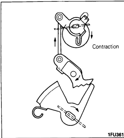
2. Before starting the engine, depress the accelerator pedal to the floor, and the fast idle cam will turn clockwise. Release the accelerator pedal, and the lever will ride on the fast idle cam and the throttle valve will open.
