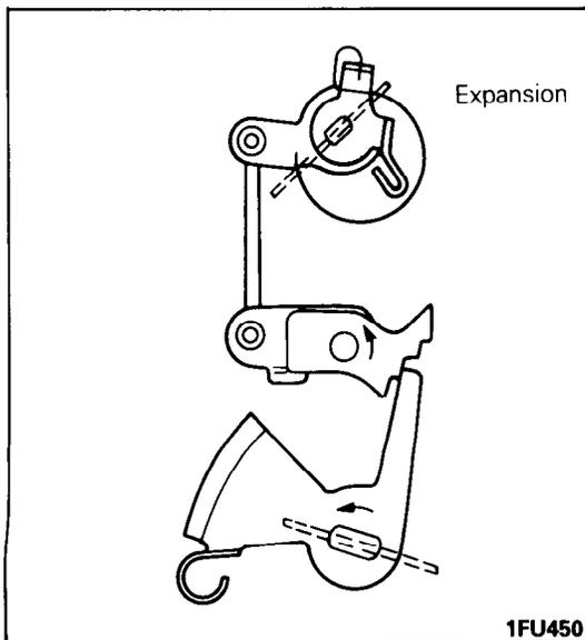
5. Depress the accelerator pedal, and the fast idle cam will turn counter-clockwise. Release the accelerator pedal and the lever will ride on the lower cam of fast idle cam and the throttle valve will close slightly, decreasing the engine speed. After warming up the engine for a while, depress the accelerator pedal and the throttle valve will be further closed. By repeating this procedure, the fast idle cam is released and the throttle valve comes to have a normal idle opening.
