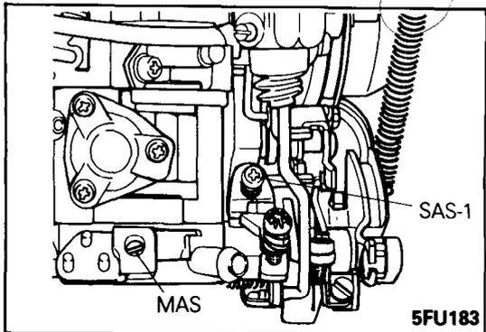
15. Set the idle CO and the engine speed to the specified value by adjusting the idle speed adjusting screw No. 1 (SAS-1) and the idle mixture adjusting screw (MAS).
