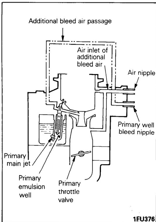
**INSPECTION OF CARBURETOR BLEED AIR PASSAGE FOR CLOGGING (INSPECTION OF CARBURETOR HIGH ALTITUDE COMPENSATION SYSTEM)**
