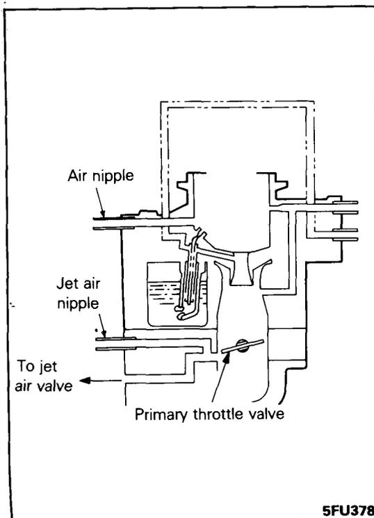
**Inspection for Clogging of Jet Air Nipple – High altitude specifications for the 49 states**
