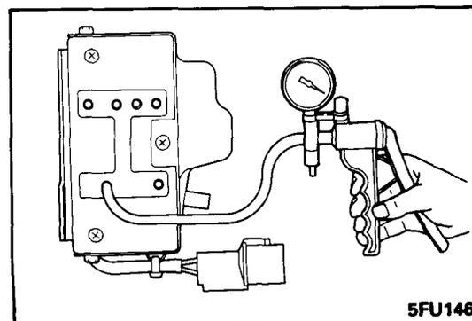
**CHECKING THE VACUUM SWITCH**
