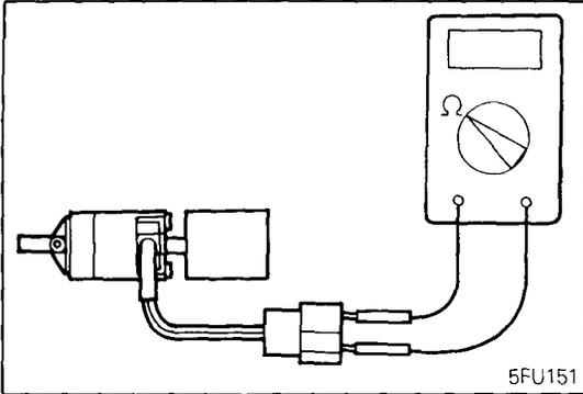
(5) Measure the solenoid coil resistance.
