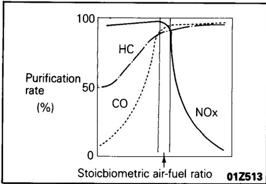
Using such characteristics, the oxygen sensor senses the oxygen concentration in the exhaust gas and feeds it to the ECU. The ECU then judges if the air-fuel ratio is richer or leaner as compared to the stoichiometric ratio and provides feedback control to adjust the air-fuel ratio to the stoichiometric ratio where the emission purification rate of the three-catalyst converter is the optimum.
