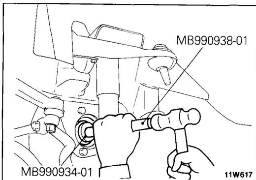
8. Press-fit the oil seal positively with the special tool and apply a thin coat of specified grease to the lip of the oil seal.
