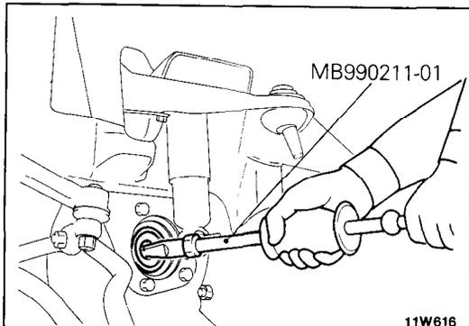
6. Remove the differential mounting bracket (R.H.) and housing tube. (Refer to 2-66, 68.)
