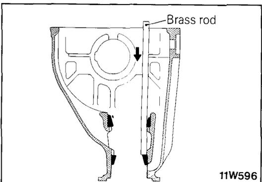
**28. REMOVAL OF DRIVE PINION REAR BEARING OUTER RACE**
