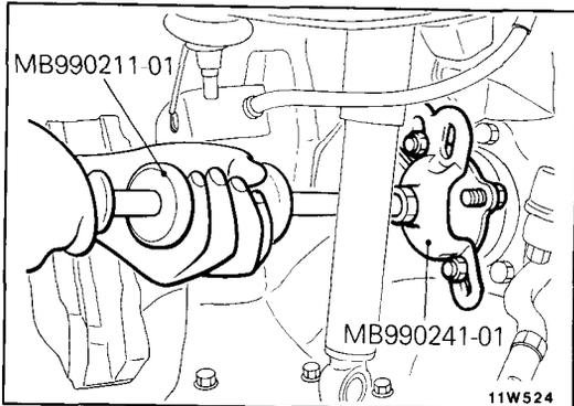
4. Remove the right drive shaft from the inner shaft assembly.
