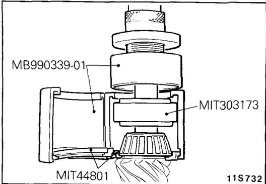
**20. REMOVAL OF DRIVE PINION FRONT BEARING INNER RACE**
