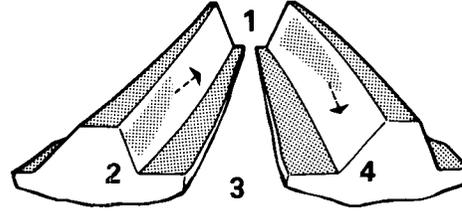
The drive pinion is positioned too far from the center of the drive gear.
