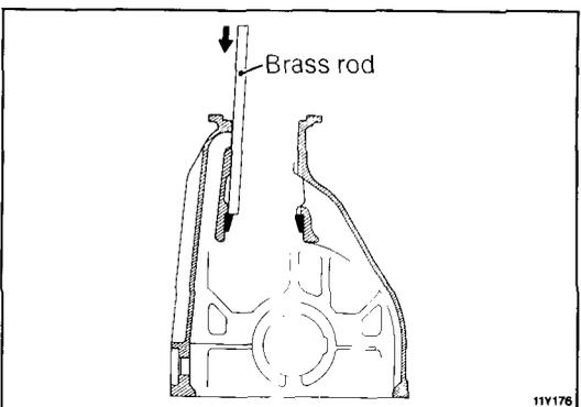
**29. REMOVAL OF DRIVE PINION FRONT BEARING OUTER RACE**
