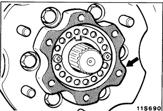
**6. INSTALLATION OF MANUAL FREE-WHEELING HUB ASSEMBLY**
