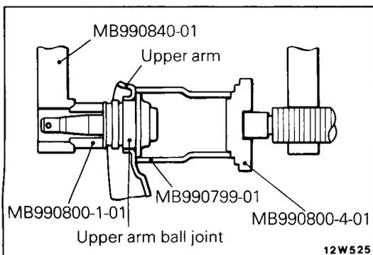
3. Press the upper ball joint out of the upper arm by using the special tools.
