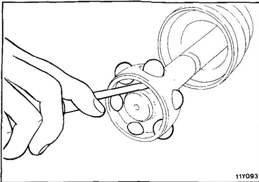
**SERVICE POINTS OF DISASSEMBLY****5. REMOVAL OF BALLS**
