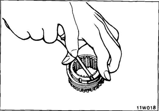
**18. REMOVAL OF SLIDE GEAR C-RING**
