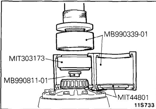
**7. REMOVAL OF SIDE BEARING INNER RACES**
