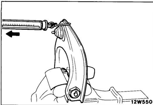
**UPPER ARM SHAFT STARTING TORQUE**
