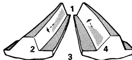
The drive pinion is positioned too close to the center of the drive gear.
