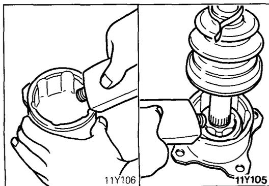
**4. INSTALLATION OF D.O.J. OUTER RACE**
