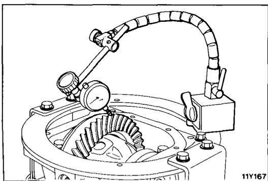
(3) Measure the thickness of the side bearing adjusting spacers on one side, select two pairs of spacers which correspond to that thickness plus one half of the clearance plus 0.05 mm (.002 in.), and then install one pair each to the drive pinion side and the drive gear side.
