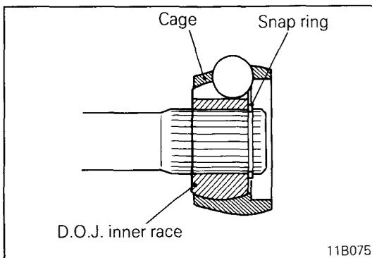
**6. INSTALLATION OF D.O.J. CAGE / 8. D.O.J. INNER RACE**
