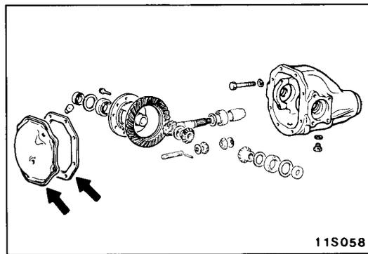
(8) Change the side bearing adjusting spacers as illustrated, and then adjust the final drive gear backlash between the drive gear and the drive pinion.
