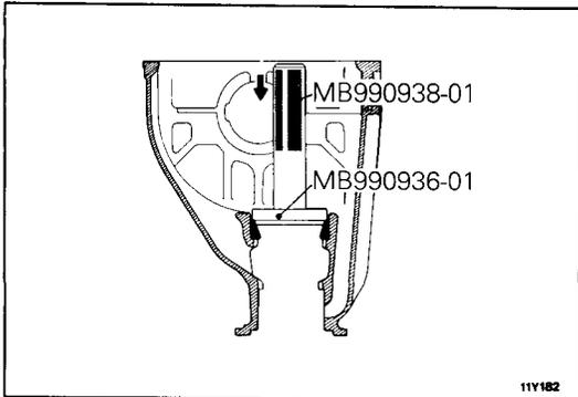
**4. INSTALLATION OF DRIVE PINION FRONT BEARING OUTER RACE**
