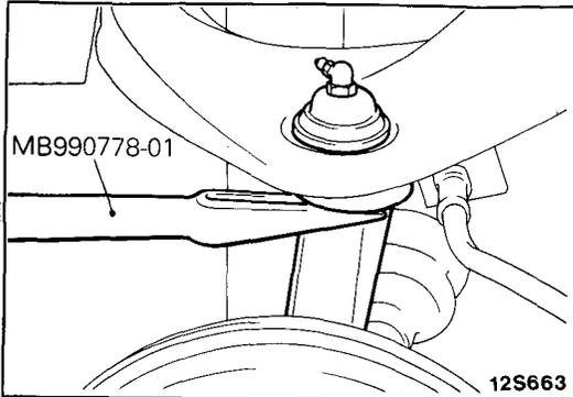
**6. DISCONNECTION OF UPPER BALL JOINT FROM KNUCKLE**
