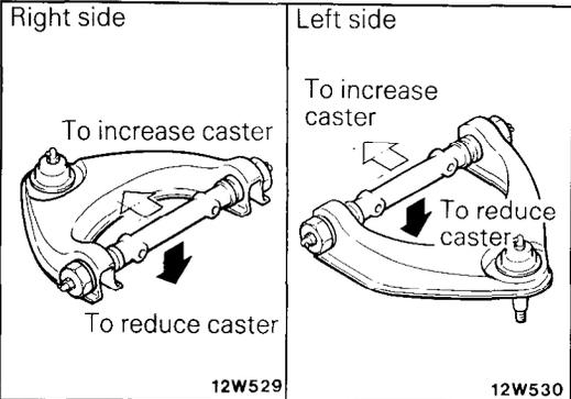
3. If caster does not meet specifications, remove the upper arm from the crossmember and then adjust by turning the upper arm shaft.
