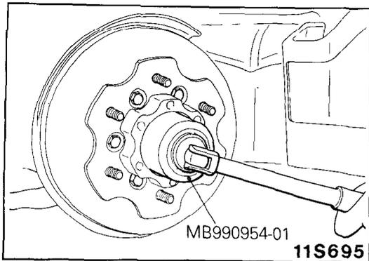
**9. REMOVAL OF LOCK NUT/10. FRONT HUB ASSEMBLY**
