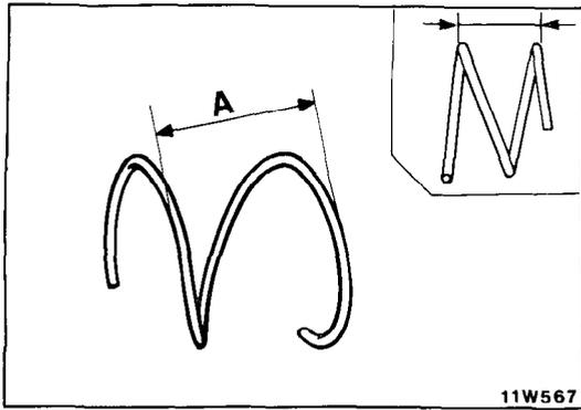
**DETERIORATION OF RETURN SPRING**
