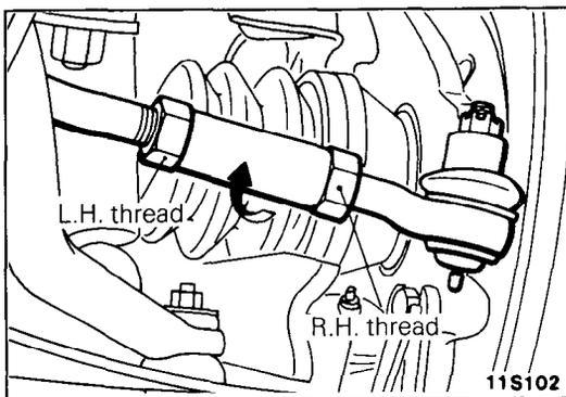
2. If the toe-in does not agree with the standard value, use the left and right tie rod turnbuckles to adjust it.
