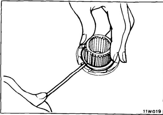
**15. REMOVAL OF DRIVE GEAR SNAP RING**
