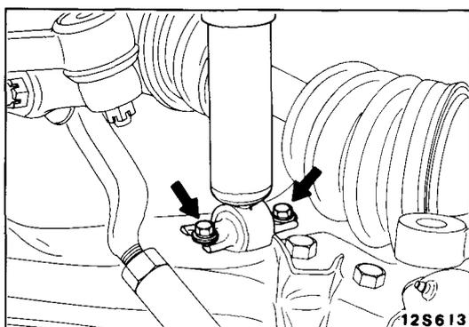
**8. REMOVAL OF SHOCK ABSORBER MOUNTING BOLTS**
