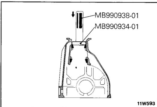
**5. INSTALLATION OF DRIVE PINION REAR BEARING OUTER RACE**
