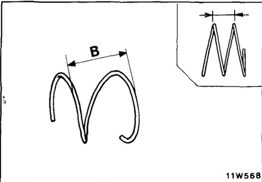
**DETERIORATION OF SHIFT SPRING**
