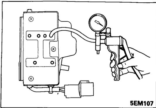
**INSPECTION OF VACUUM REGULATOR VALVE (VRV)**
