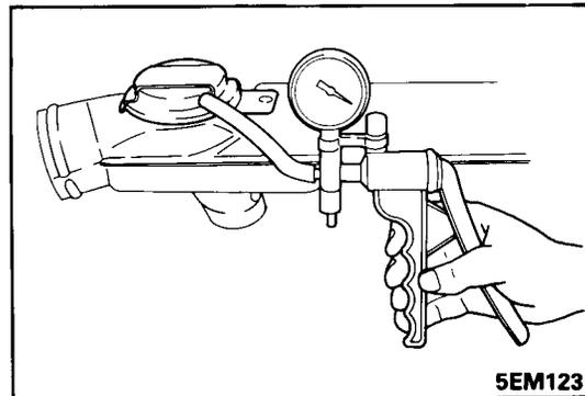
**INSPECTION OF AIR CONTROL VALVE AND THERMO SENSOR**
