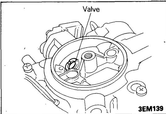
**INSPECTION OF MIXTURE CONTROL VALVE (MCV)
