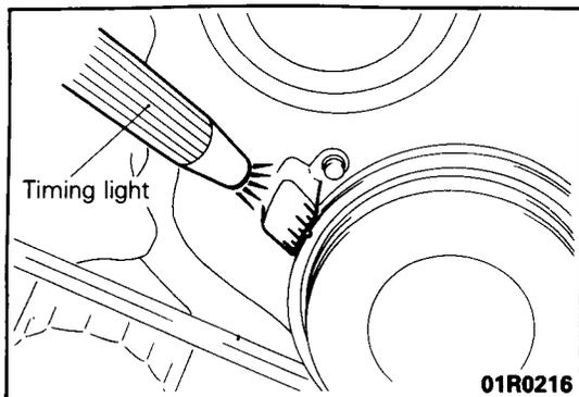
(6) Run the engine at idle and check ignition timing.
