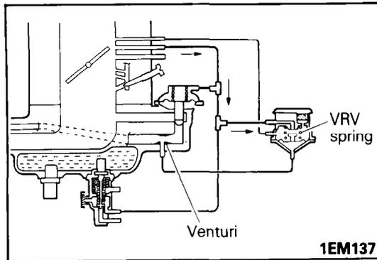
When the venturi pressure drops to near the atmospheric pressure, the VRV opens to allow the E port vacuum to escape to atmosphere. Then, the EGR valve closes. By repeating this cycle (closed loop control), EGR flow rate proportional to the intake air volume can be obtained.
