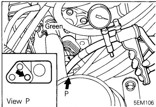
**INSPECTION OF EXHAUST GAS RECIRCULATION (EGR) SYSTEM**
