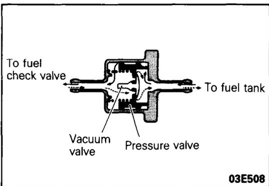
**OVERFILL LIMITER (TWO-WAY VALVE)**
